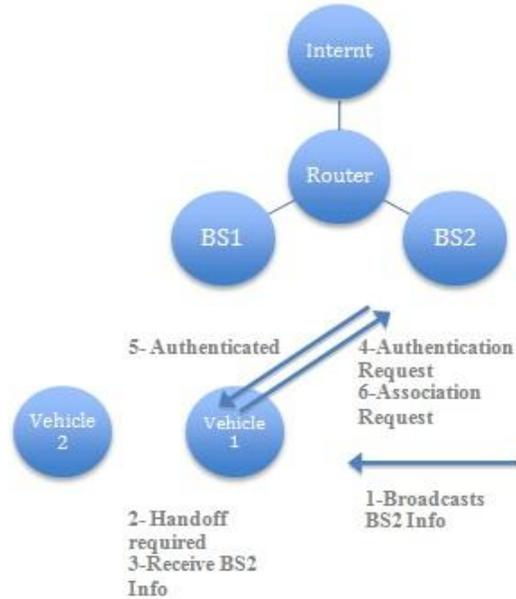
Fig. 4 Schematic View of Enhanced Velocity-Based Handoff Process
